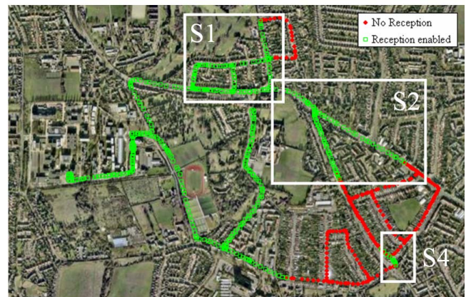
Figure 13. MISO reception along the Route B. The squares indicate the route sectors where a major reception gain was observed.
