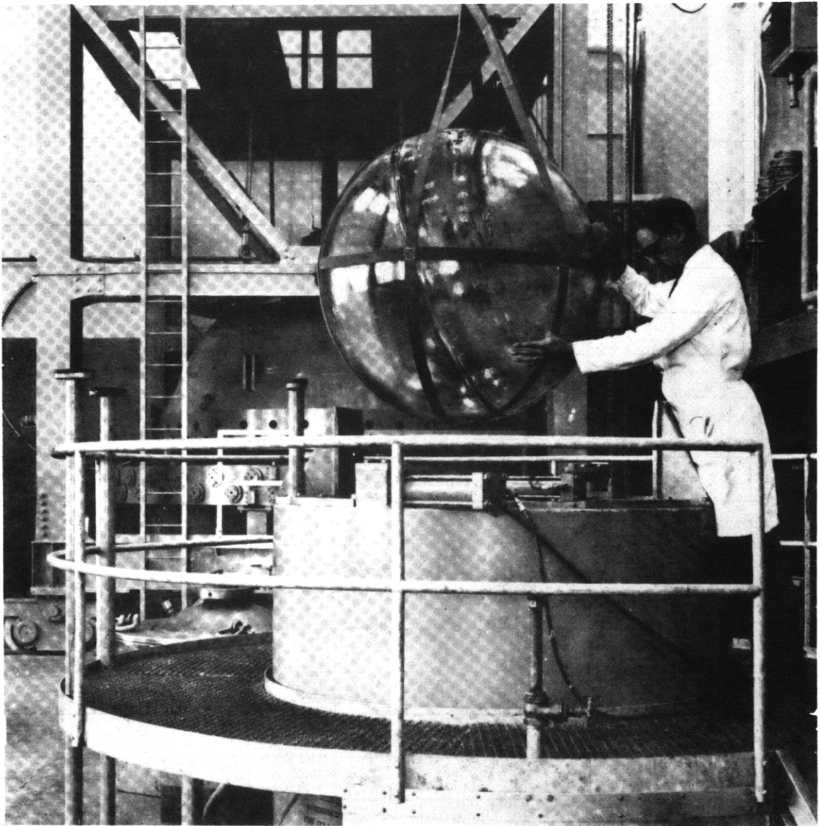
Figure 23 - 44 Inch Diameter Fusion Sealed Annealed Glass Sphere
