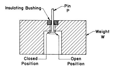
Figure 2 - Large scale detail of pin-contact of microphonic switch
