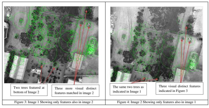
Now that the two images have features that match and the exact location within the image of these points is know the two images can now be combined. To do this the images must undergo further analysis to find the areas of the images that will be overlapping. MATLAB provides a function 'estimateGeometricTransform' that determines any changes needed to the orientation.
