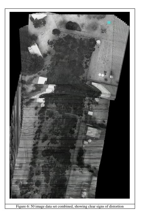
Expanding the data set to include all images produces the results similar to those in Figure 6. Investigation into the results of figure 7 show that in addition to the incorrect overlapping; there is also added discontinuation of images being experienced.
