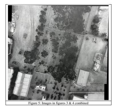
Extending the data set to include a significantly larger area to analyse is done by following the same process while looping for each image. The algorithm is able to stitch together a larger set of images however a major issue is evident. This problem is multiple images are overlapping incorrectly as seen at the top of Figure 6. The possible reasons for this are incorrect feature detection or possible incorrect geometric transforms.
