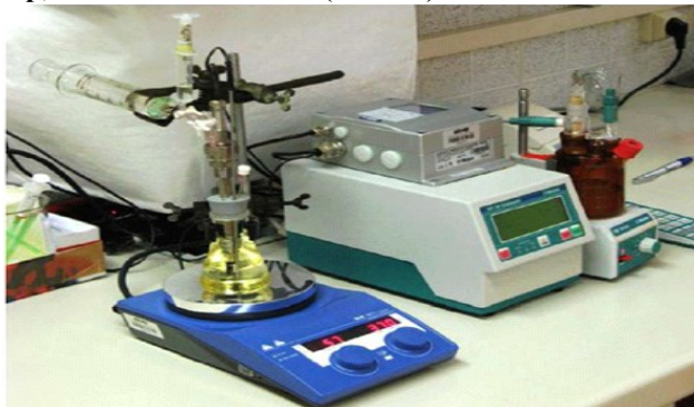
Figure 1: A link test setup, left: moisture sensor (Delta T) and Metrohm 756 Karl Fischer Coulometer.
