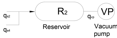
Fig. 7. The scheme of the process of releasing compressed air in the improved system
