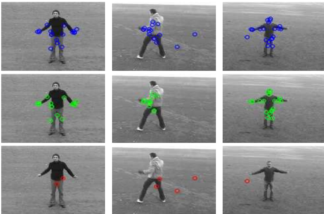
Figure 4.3: Key points detected by BRISK detector on sample frames from KTH dataset are shown in the first row. The second row shows the candidate key points for description and the last row shows the eliminated points due to insignificant motion. Sample actions are Hand clapping (first column), Boxing (second column), Waiving (third column)
