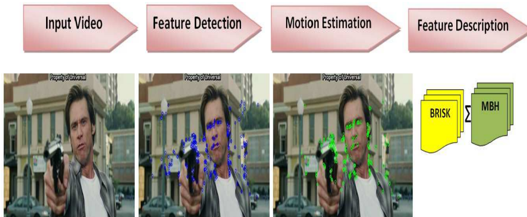
Figure 4.1: Proposed Framework for local feature extraction, which consists of key point detection, motion estimation followed by appearance and motion description.
