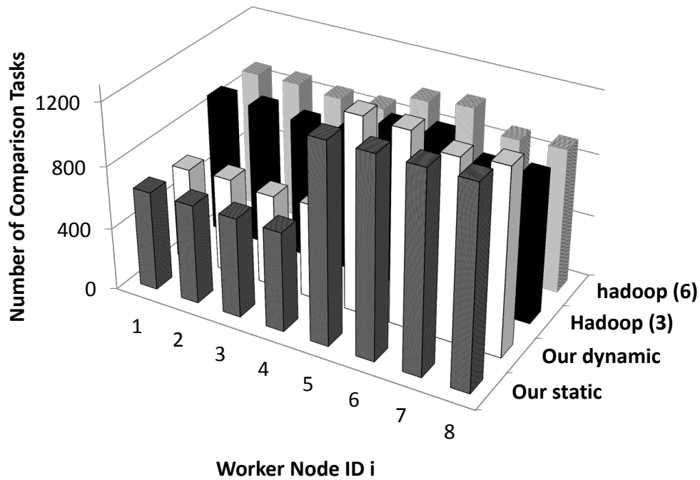
Figure 7.11: The number of comparison tasks completed on each node. Nodes 1 to 4 have twice the computing power of Nodes 5 to 8.
