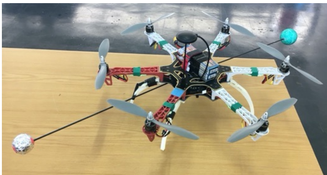
Figure 3.21: Polystyrene balls used to help with the direction of the aircraft.
