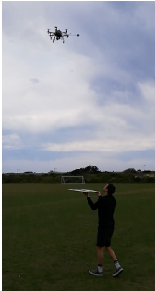
Figure 7.7: The multirotor aircraft hovering above the ArUco marker when a person held the marker
