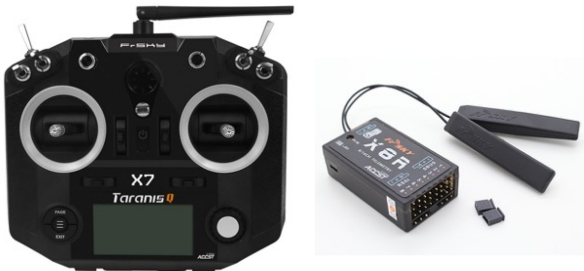
Figure 3.10: (a) FrSky Taranis Q X7 transmitter (GetFPV, 2019) (b) FrSky X8R receiver (PorcupineRC, 2019)
