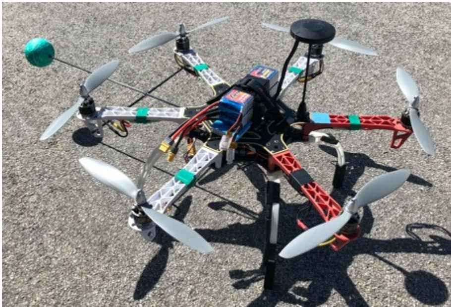
Figure 3.22: Modification of keeping the tail polystyrene ball and supporting the rod
