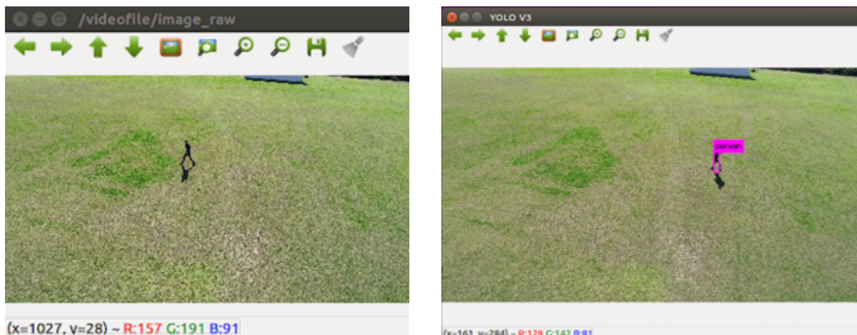
Figure 6.7: (a) Video of a person walking that was published by the video_stream_opencv package (b) bounding box that was formed using the darknet_ros package
