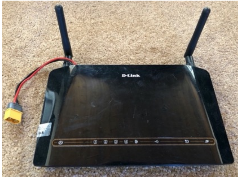
Figure 3.20: Modified D-Link DSL-2750U modem router
