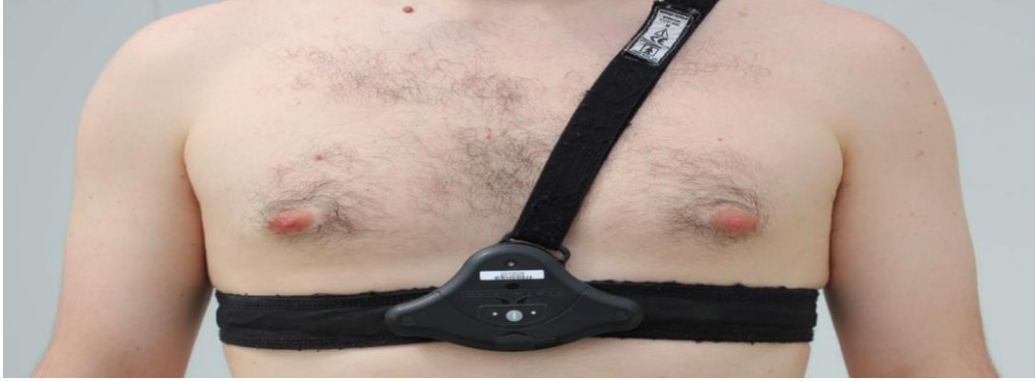
Figure 3.12: Wearable Smart Belt for Remote Monitoring of Physiological and Behavioural Status (Banos et al. , 2014)
