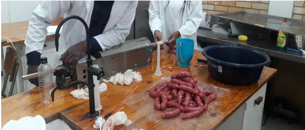
Figure. 6 Casing attached to the filler
