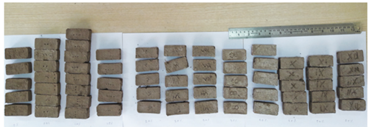
Figure 2. Different batches of bricks with HEP waste bricks.
