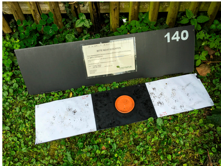
Figure A1. Footprint tunnel with removable plate in front, showing hedgehog footprints on them. Two paper sheets and two brushes of ink are applied to it. A spoon of bait is placed in the brown plate. © Thomas Massie/stadtwildtiere.ch.
