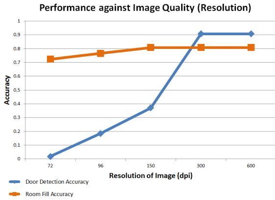
Figure 5: Plot of room and door detection accuracy against bitmap resolution
