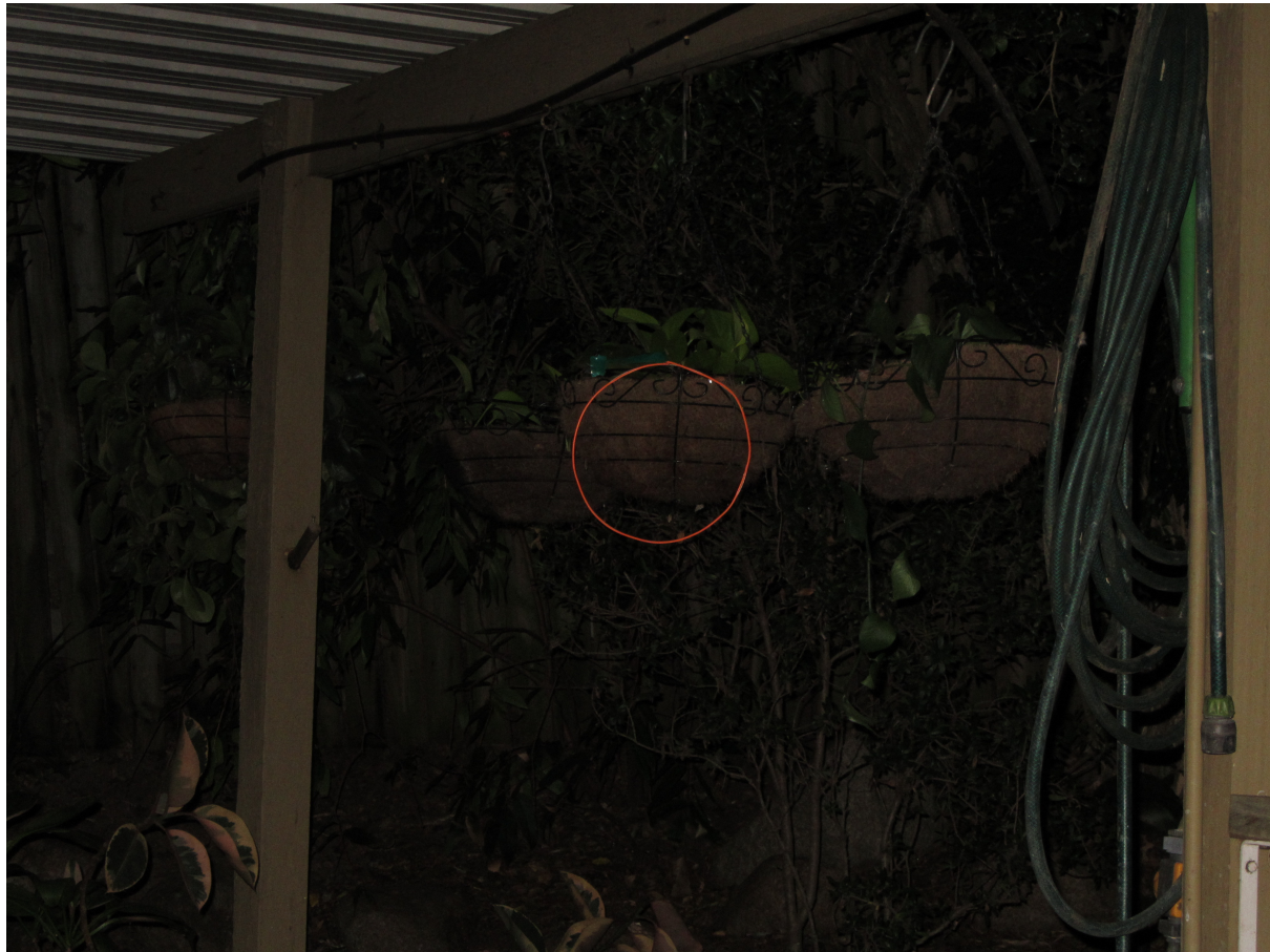
Figure 9. A simulated Rim of Fire made from a 1 m electroluminescent (EL) wire 2 mm in thickness formed into a circle 25 cm in diameter. The inverter, and part of the EL wire are hidden amongst the leaves of the plant in the hanging basket.
