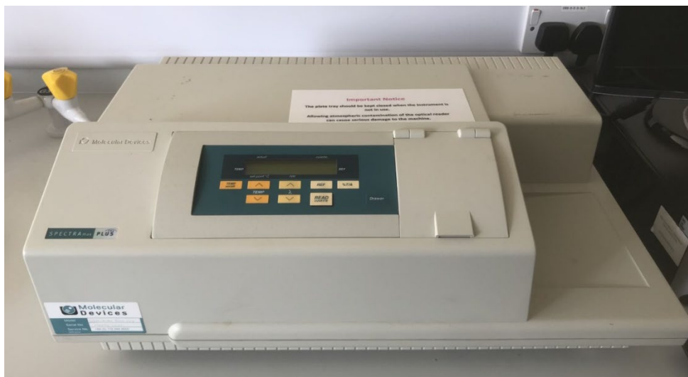
Figure 2. 26: Digital image of a SpectraMax Plus 384 Microplate Reader.
