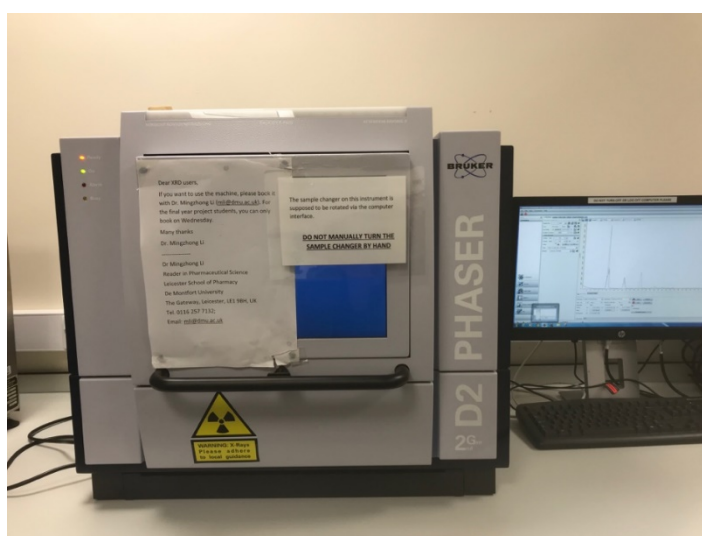
Figure 2. 21: Digital image of a Bruker 2nd Generation D2 Phaser.
