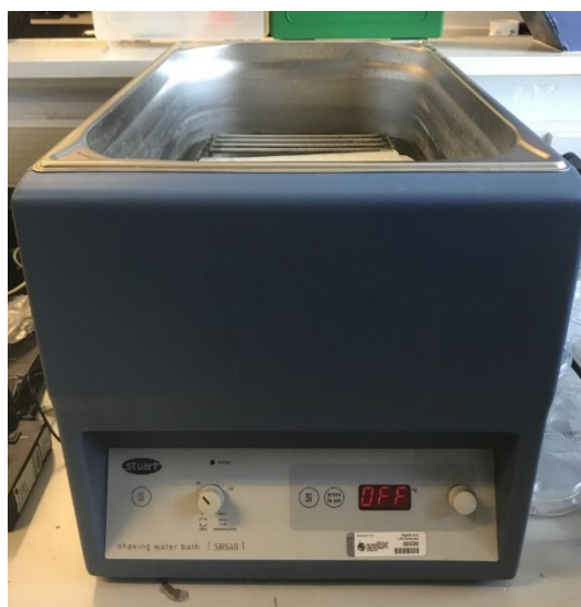
Figure 2. 24: Digital photo of a Stuart SBS40 Shaking water bath.
