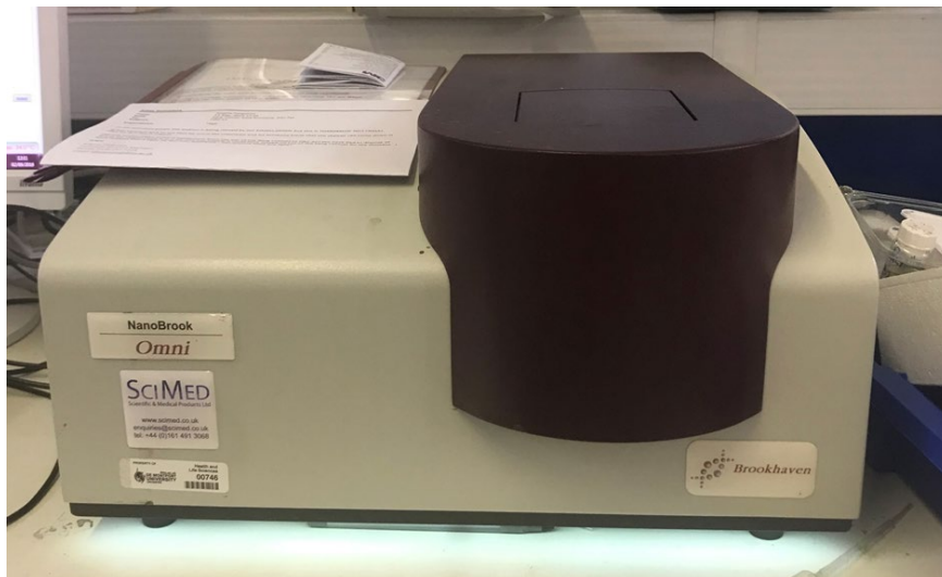
Figure 2. 23: Digital image of a Brookhaven NanoBrook Omni zeta potential analyser.
