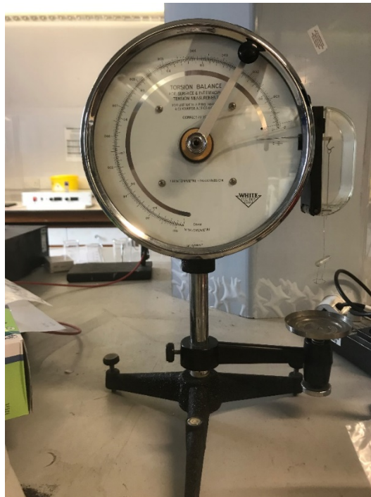
Figure 2. 14: Digital image of a White Electrical Instrument Co. OS torsion balance.
