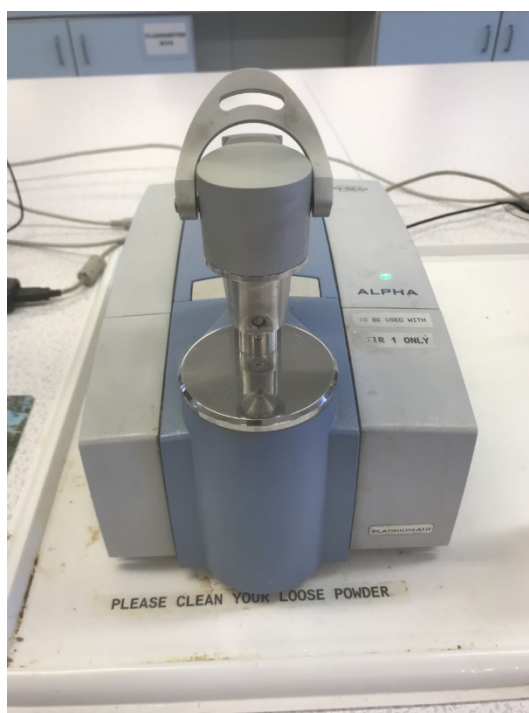
Figure 2. 20: Digital image of Bruker FTIR Platinum-ATR spectrophotometer.
