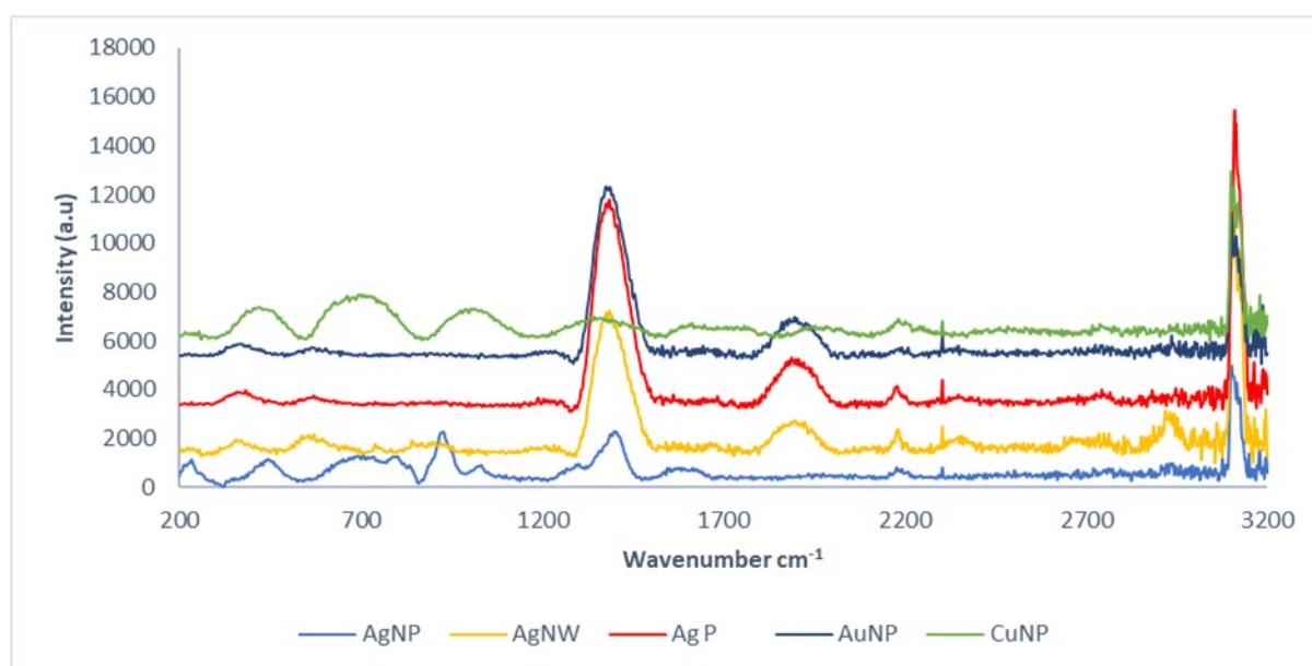
Figure 3. 5: Raman spectra of synthesised metallic nanoparticles; AgNP, AgNW, AuNP, AgP and CuNP.
