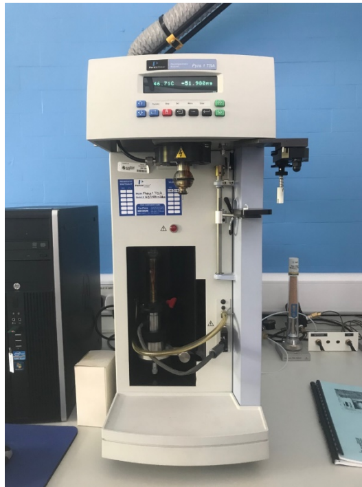
Figure 2. 19: Digital image of a PerkinElmer Pyris 1 TG analyser.
