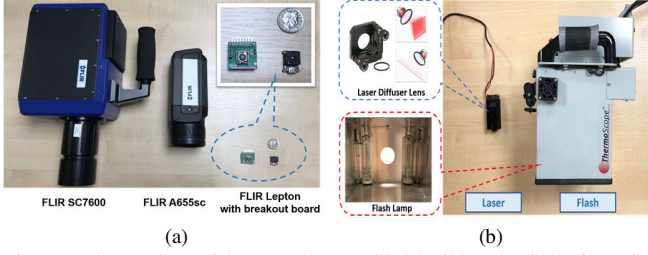
Fig. 3. (a) Comparison of the FLIR lepton with SC7600 and A655sc for active thermography. (b) Comparison of the laser and flash excitation sources
