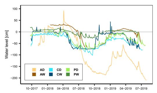
**Figure 5.** Course of water levels in the study sites over the study period. Water levels are given relative to ground surface and were measured with SEBA Dipper PT (SEBA Hydrometrie) or CS457 connected to CS1000 datalogger (Campbell Scientific; the latter in the alder forest sites).
