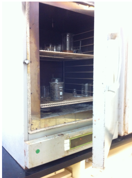
Figure 5.5: Soil sample is dried in the oven determine soil moisture content
