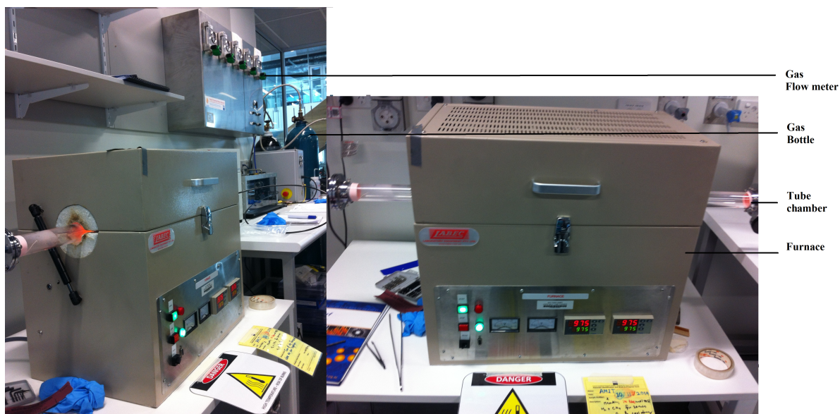
Figure 6.5: Experimental setup for the process of graphene deposition on copper process
