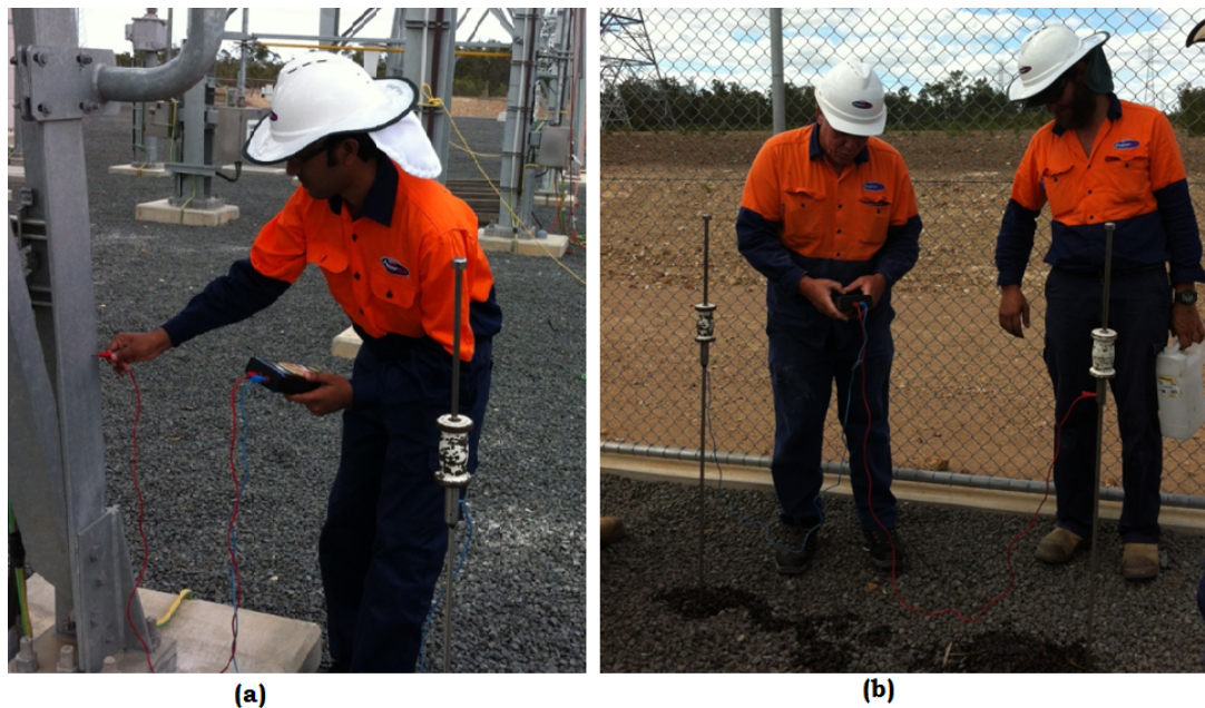
Figure 2.11: (a) Touch voltage measurement (b) Step voltage measurement
