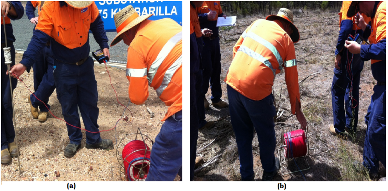
Figure 2.13: (a) EPR measurement near substation fence (b) EPR measurement a distance from the substation
