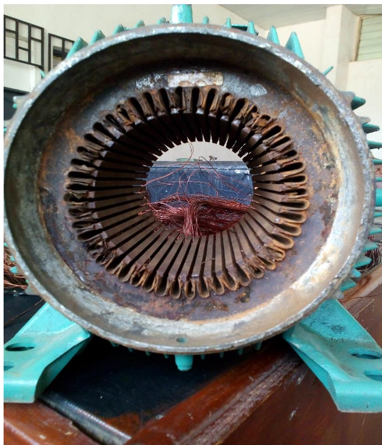
Fig. 3.25 Pictorial view of the stator without the windings
