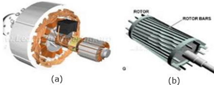
Fig. 3.2 The rotor of an AC machine (a) coiled rotor (b) squirrel cage rotor Source: Benoit et al. (2012)
