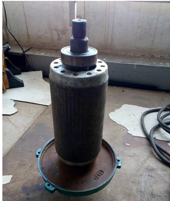
Fig. 3.26 Pictorial view of squirrel cage rotor of the induction motor
