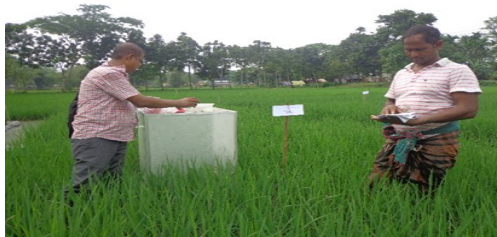
Plate 2. Collection of gas sample from paddy field.
