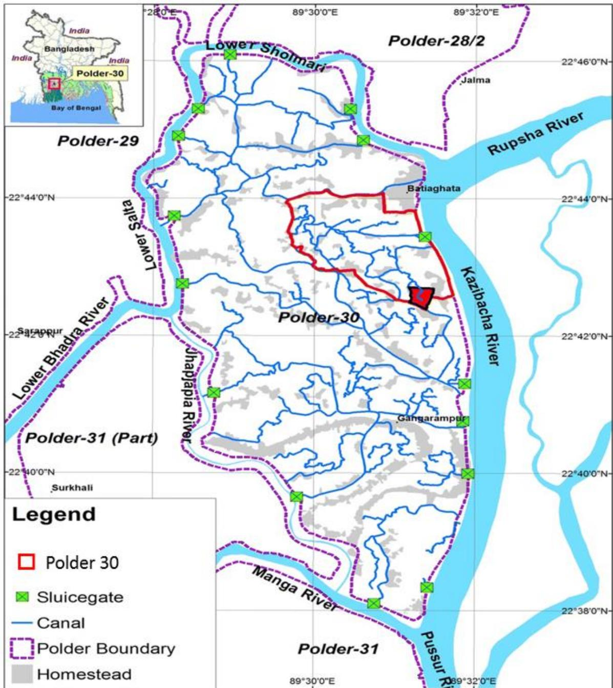
**Fig. 2.2.** Plan view of a typical polder in the coastal zone of Bangladesh (Yadav et al., 2019)
