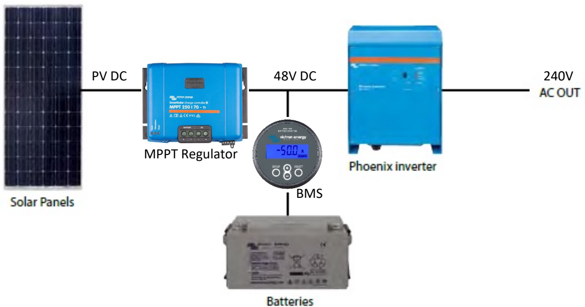
Figure 9:PVRO Basic Electrical Layout
