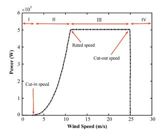
Figure 4. Wind power curve vs. wind speed.
