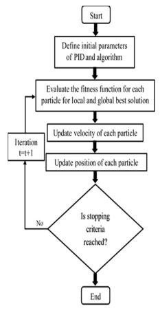
Figure 9. Flow chart of the PSO algorithm.
