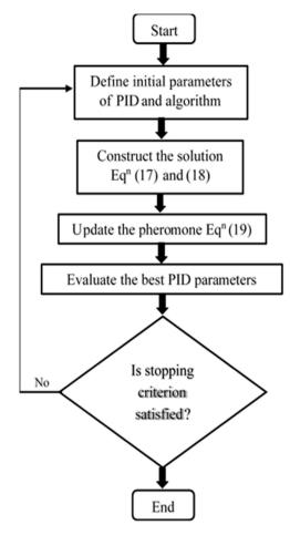
Figure 7. Flow chart of the ACO algorithm.
