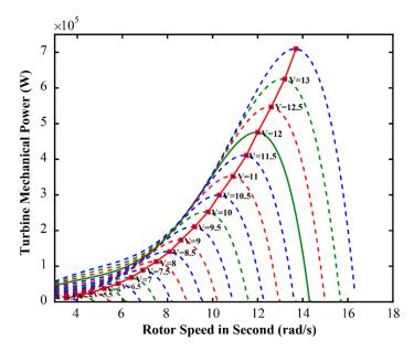
Figure 3. Turbine mechanical power curve vs. rotor speed under variable wind speeds.
