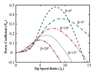
Figure 2. Power coefficient vs. tip speed ratio for different pitch angles [27].
