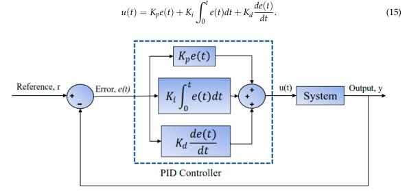
**Figure 5.** A typical block diagram of a proportional–integral–derivative (PID) controller with feedback loop.
