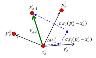
Figure 8. Particle swarm optimization (PSO) algorithms [36].
