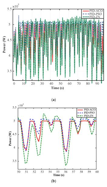
Figure 14. (a) Output wind power generation by the proposed controller; (b) Zoomed figure region.
