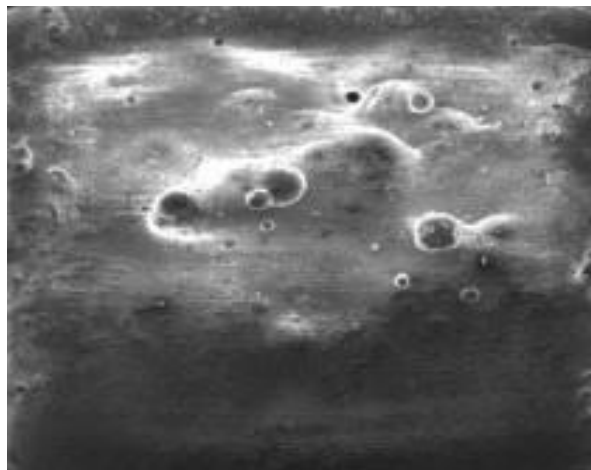
Figure 8. Balling microstructures formation in aluminium alloys during the SLM process. 35
