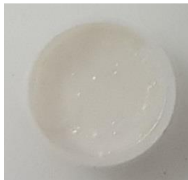
Figure 4-9: Appearance of Chlorella ash in TGA crucible after ashing at 1000 °C in air.
