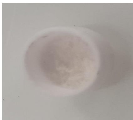
Figure 4-14: Residue from oxidation of whey protein in TGA at 600 °C in presence of air.
