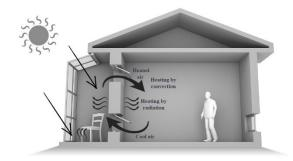
Figure 5, Sunspace indirect heating mechanisms
