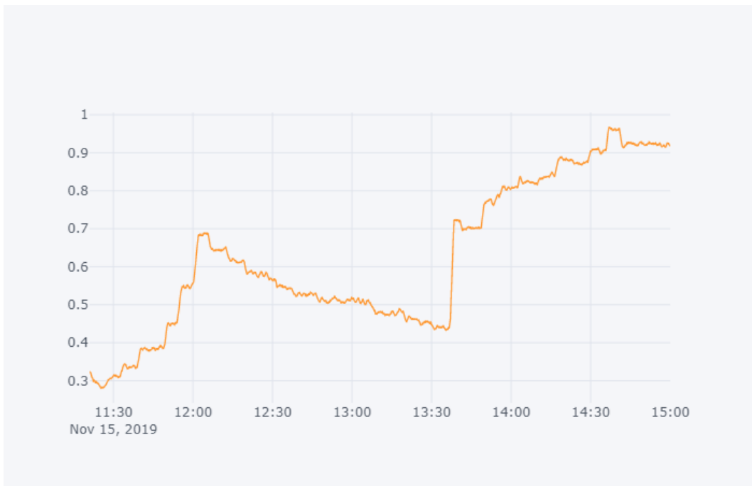
Figure 9.6 Trend log for the fan's outlet static pressure (in. WC).
