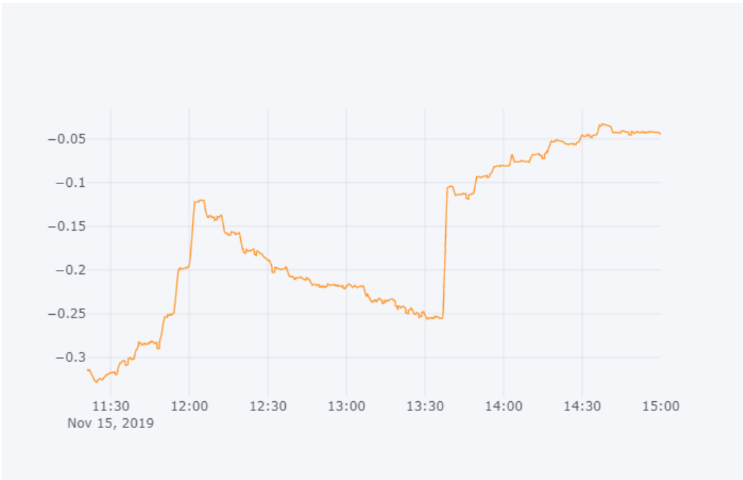
Figure 9.5 Trend log for the fan's inlet static pressure (in. WC).
