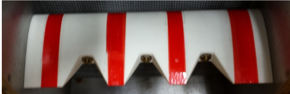
Figure 3-3: Atomizers arrangement in the wind tunnel [82].
