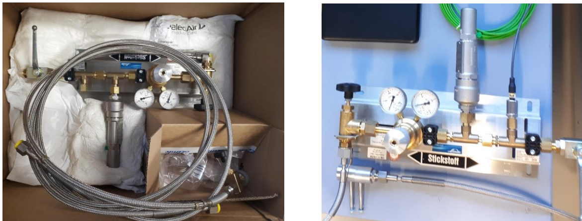
Figure 3-14: Pressure control unit manufactured and assembled by Linde Group.
