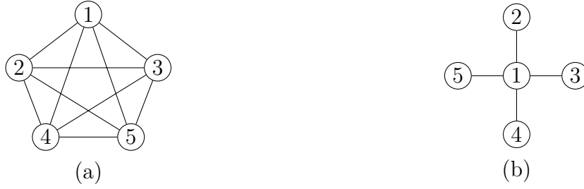
Figure 2.4: Two network topologies in which the leader is connected to all agents.
