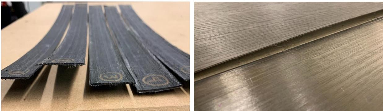
**Figure 7.** Distortion of the composite laminate during and after the process
