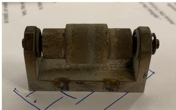
**Figure 21.** Consolidation roller of AFP setup
