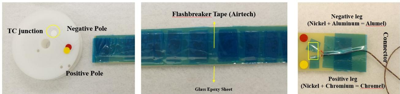
**Figure 29.** Fast-response K-type thermocouple assembly
