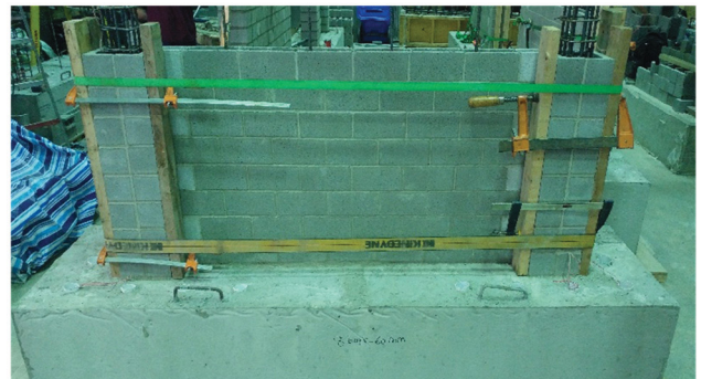
(6) Strapping & grouting of 1 st one-third
