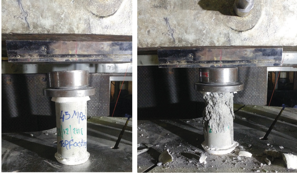
Figure A.24 Testing of the bottom and top footings' concrete
