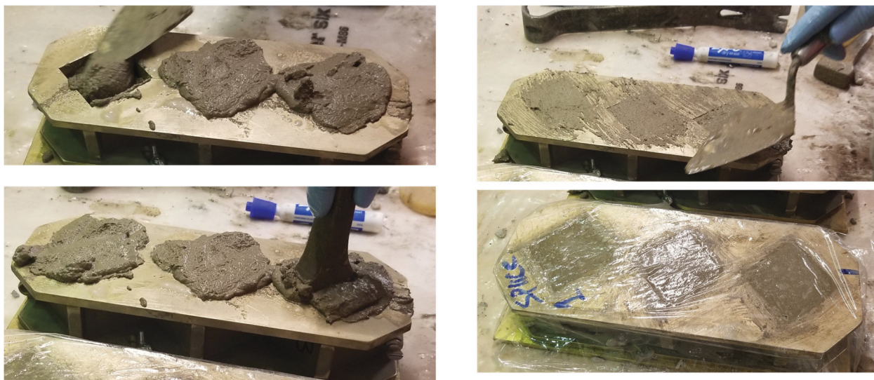
Figure A.19 Sampling of Type S mortar cubes
