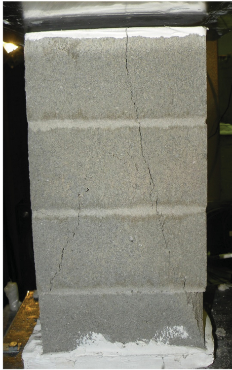
Figure A.26 Typical final damage states of tested web (stretcher blocks) prisms
