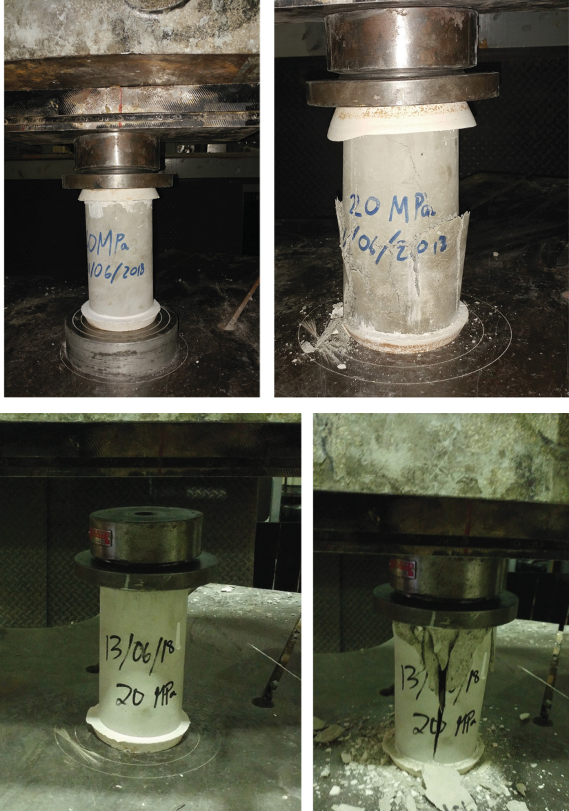
Figure A.21 Testing of the grout cylinders
