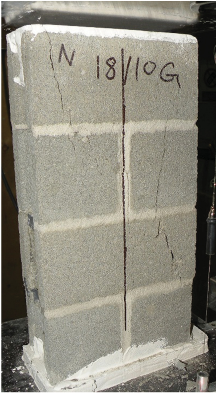
Figure A.26 Typical final damage states of tested web (stretcher blocks) prisms
