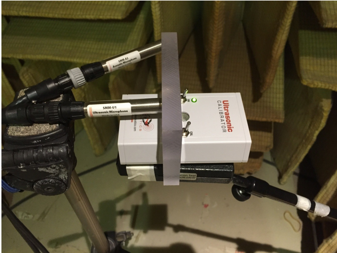
Figure 3.12: Calibration of the SMM-U1 ultrasonic microphone in an anechoic chamber. The professional calibrator (Wildlife Acoustics Inc.) produced a 40 000 Hz sine wave of 75 \pm 3 dB (re: 20\mu\text{Pa} ). It was mainly used to assess the quality of the microphone rather than precisely indicating the sensitivity of the microphone. A “sensitivity” above -38dBV meant that the microphone was still of good quality. Since this was the case, we based this microphone’s sensitivity on the chart provided by Wildlife Acoustics (Figure 3.13 below) for the sound pressure levels adjustments.
