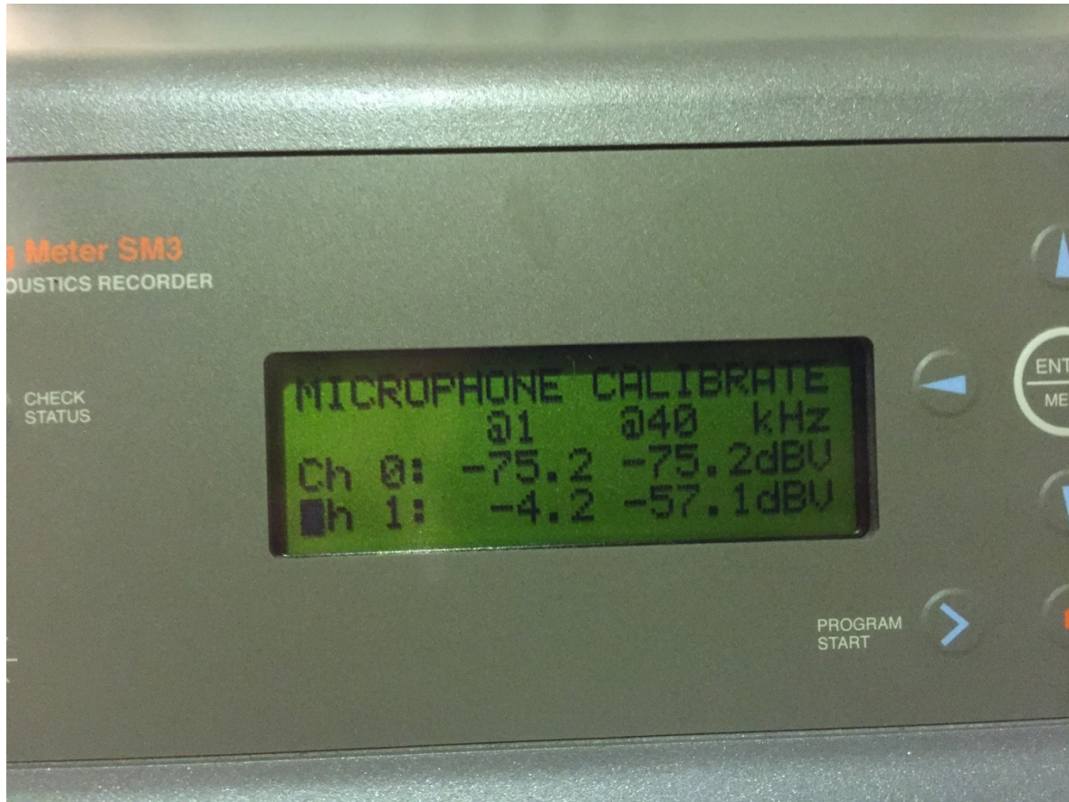
Figure 3.14: Example of the calibration mode of the SMM-A2 acoustic microphone with the calibrator producing a sine wave of 1 000 Hz. The microphone is represented by the channel 1, and under the column @1 kHz the sensitivity is indicated (-4.2 dBV, which was later applied to correct the sound level recorded). This microphone was not sensitive to 40 000 Hz, therefore any result under that column was disregarded. The channel 0 represents the SMM-U1 ultrasonic microphone, but it was not sensitive to 1 000 Hz sound waves, and therefore could not be tested for this particular calibrator (shown in Figure 3.11). It was tested with a professional ultrasonic calibrator (shown in Figure 3.12).
