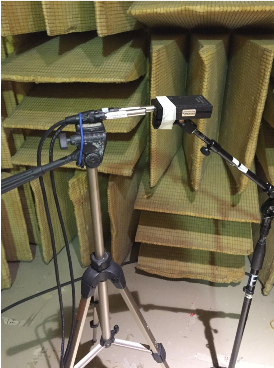
Figure 3.11: Calibration of the SMM-A2 acoustic microphone in an anechoic chamber. The professional calibrator produced a 1 000 Hz sine wave of 94 dB (re: 20 \mu Pa).
