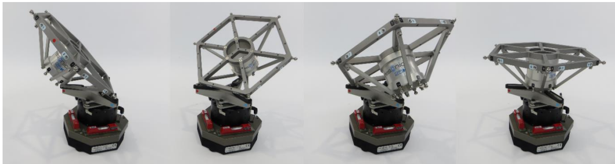
Figure 11: Different positions of the carrier platform on the air-bearing pendulum
