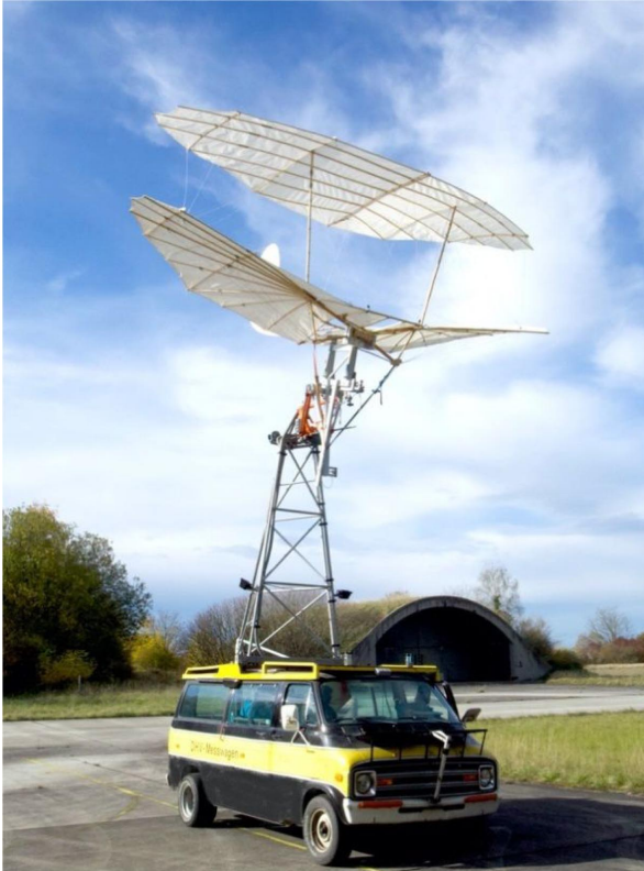
Fig. 3 Balance force and moment measurements with the Lilienthal glider mounted on the supporting structure of the test vehicle of the German Hang Gliding Association.
