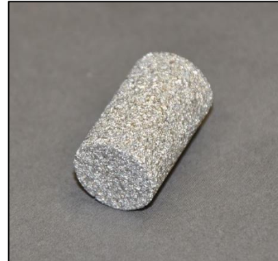
Fig. 10: Sintered stainless steel porous material
