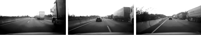
Fig. 10: Images of the front-facing camera for the start (left), the point in time with the maximum normalized distance (middle) and the end of the extracted lane-change maneuver.
