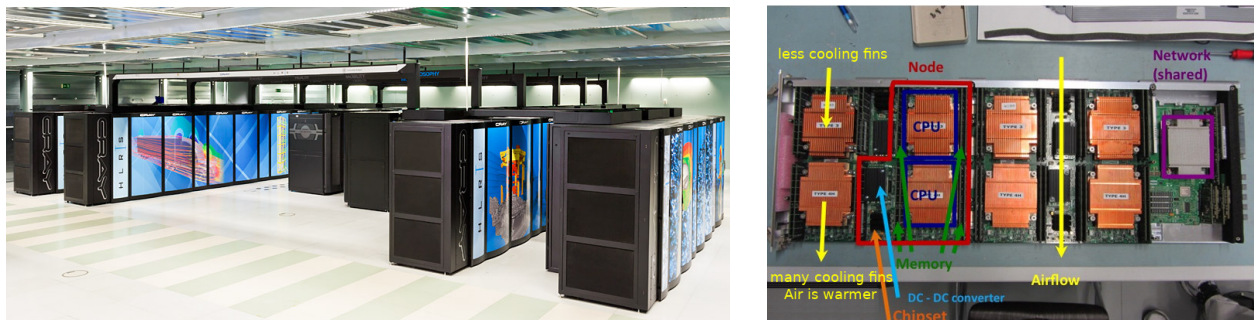
Figure 4.6: Supercomputer „Hazel Hen“ (Cray XC40) at HLRS and its blade with four compute nodes
