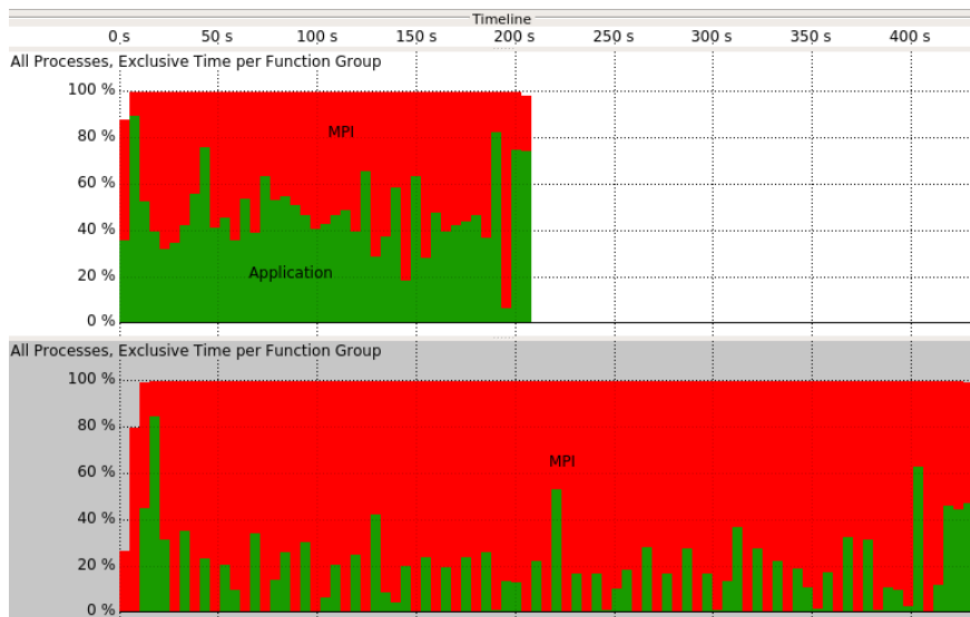
Figure 5.12: Comparing the runtime spent in the functions of the application (green) against the time spent in MPI calls (red).
