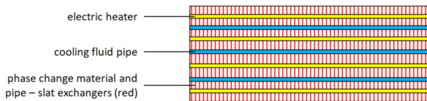
Figure 11. Conceptual design of the thermal energy storage prototype using paraffin wax for heating an electric bus from Fraunhofer and Konvekta [40].
