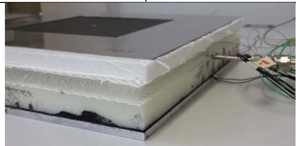
Different layers of integrated ITO with Al6065 plate at bottom and INCONEL cover plates on top
