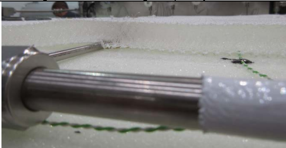
Purge feedlines going through gas permeable spacer fabric
