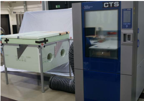
Figure 20: Climatic chamber in preparation and control unit for ITO tests at DLR cryogenic lab Bremen
