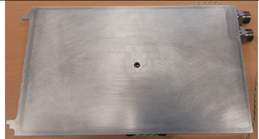
Top side of aluminum liquid nitrogen container
