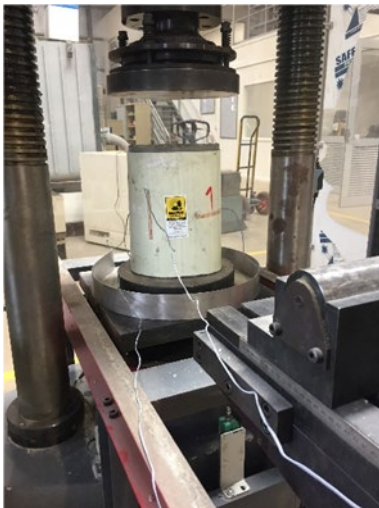
Figure 5. Sample in the compression-testing machine
