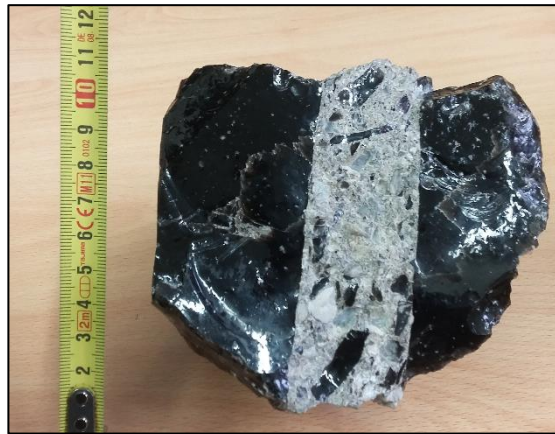
Figure 4. 6 Picture of a fracture in rhyolitic obsidian from Volcán Chaitén. This sample is from a larger bomb erupted from the 2008 dome. The fracture is filled with a polydisperse distribution of volcanic ash and glass fragments. This geometry is the basis for our calculated sequestration efficiencies.
