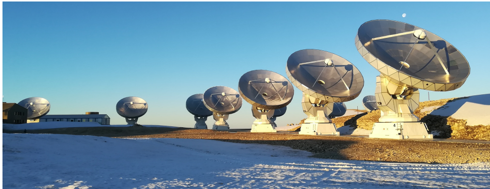
Figure 1.8: NOEMA (Northern Extended Millimeter Array). Ten of the future twelve 15-meter dishes. Credit: IRAM.
