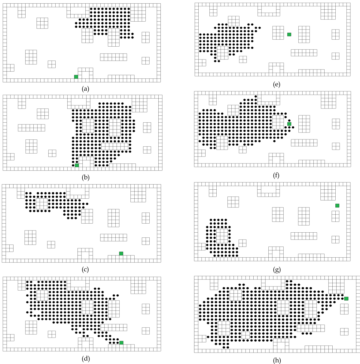
Figure 9. The results of simulated ML-PSO and basic PSO algorithms in Environment 3 with 14 static obstacles in 100 runs. Explored space is represented by the black dots and the target is shown by the green square. (a) The simulation result of basic PSO algorithm with target point 1. (b) The simulation result of ML-PSO with target point 1. (c) The simulation result of basic PSO algorithm with target point 2. (d) The simulation result of ML-PSO with target point 2. (e) The simulation result of basic PSO algorithm with target point 3. (f) The simulation result of ML-PSO with target point 3. (g) The simulation result of basic PSO algorithm with target point 4. (h) The simulation result of ML-PSO with target point 4.
