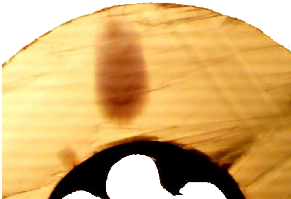
(c) A large vented water tree growing in XLPE.
