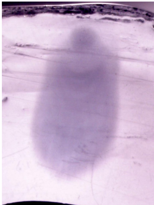
(a) Vented water tree from 2.5c after staining with methylene blue.
