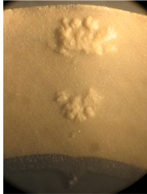
(b) Bow tie water tree in EPR.
