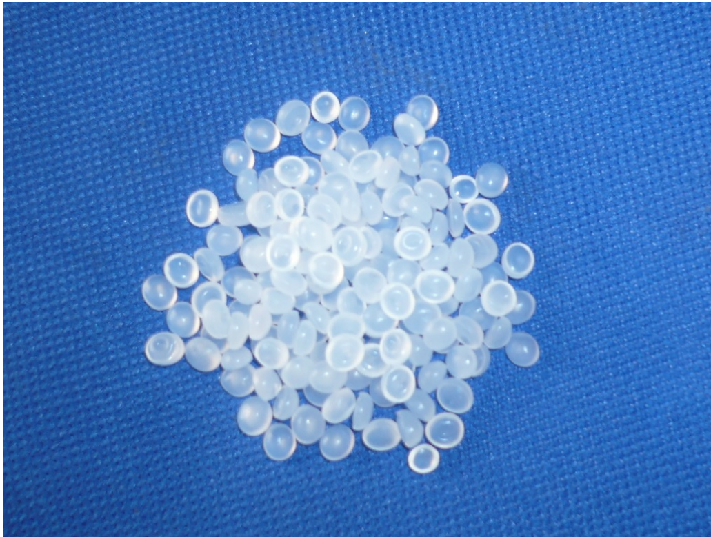
Figure 2.1: Polyethylene pellets, as used in the manufacture of XLPE.
