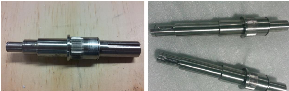
Figure 64. Original motor shaft (left image) and the modified motor shafts (right image).
