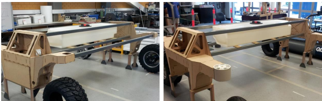
Figure 40. Mock-up vehicle assembly reviewing the construction of the implement section.
