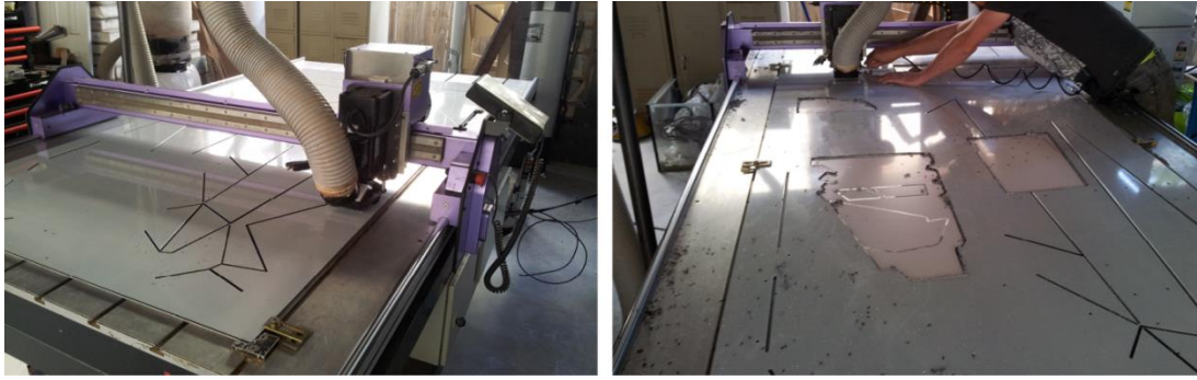
Figure 61. Routing the 45° grooves into the Dibond sheet and then cutting the outside profile.
