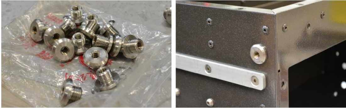
Figure 47. The machined stainless steel inserts are installed into a battery box, providing a solid fastening point when mounting to the side unit. Slide rails are also integrated to aid in the positioning and load retention.
