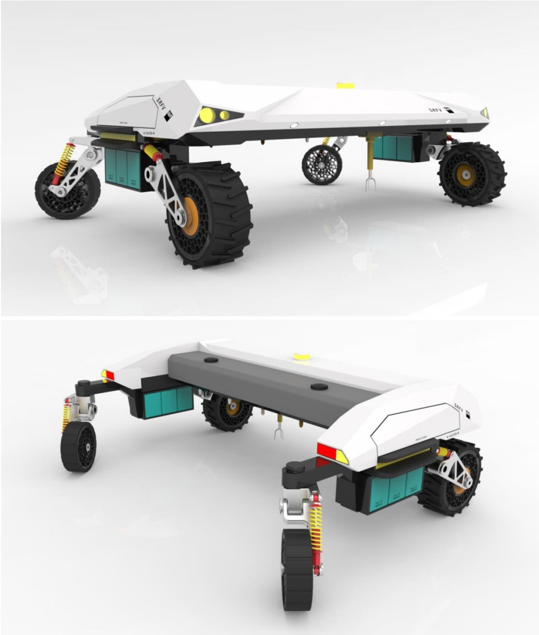
Figure 28. Concept rendering of the vehicle showing the development of the configuration, placement of the wheels, power storage, suspension and direction for the vehicle aesthetics.
