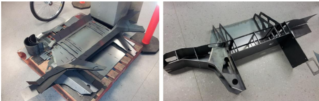
Figure 36. Pallet load of laser cut mild steel components and a test assembly of the side unit.
