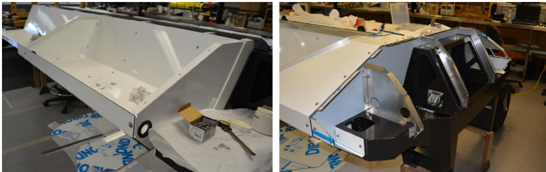
Figure 59. Attachment brackets for the covers mounted to the implement and chassis section.
