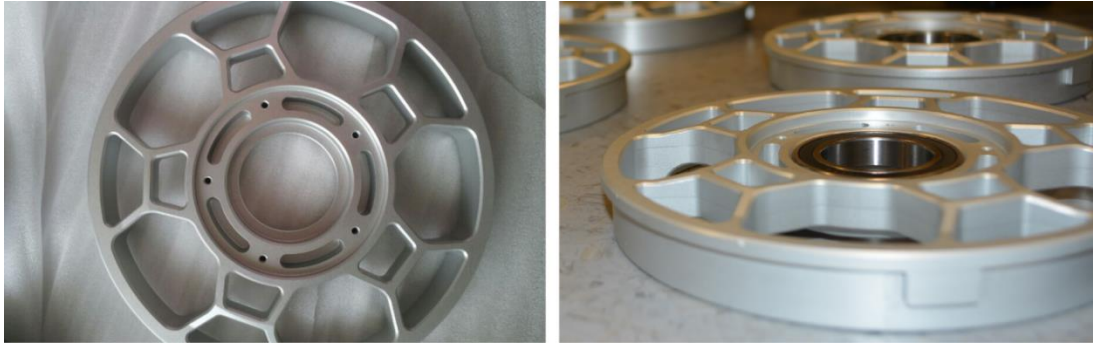
Figure 56. The CNC machined bearing housing prior to having the bearing fitted, and the final assembly with the 40mm bearing seated in the machined pocket.
