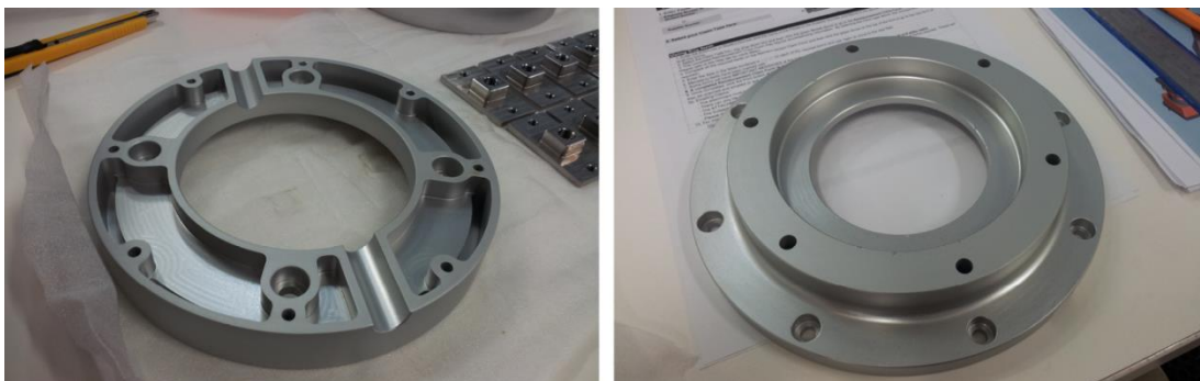
Figure 65. Custom mounting plates for attaching the motor/gearbox.
