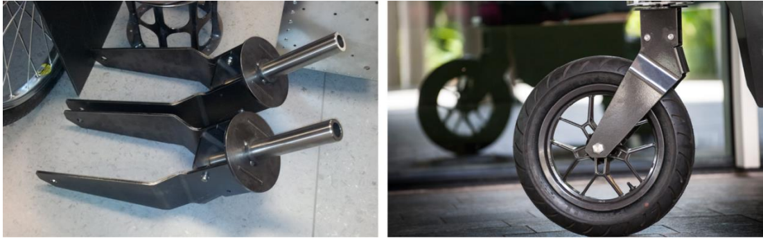
Figure 55. The caster frame during fabrication and mounted to the vehicle showing the vertical offset.
