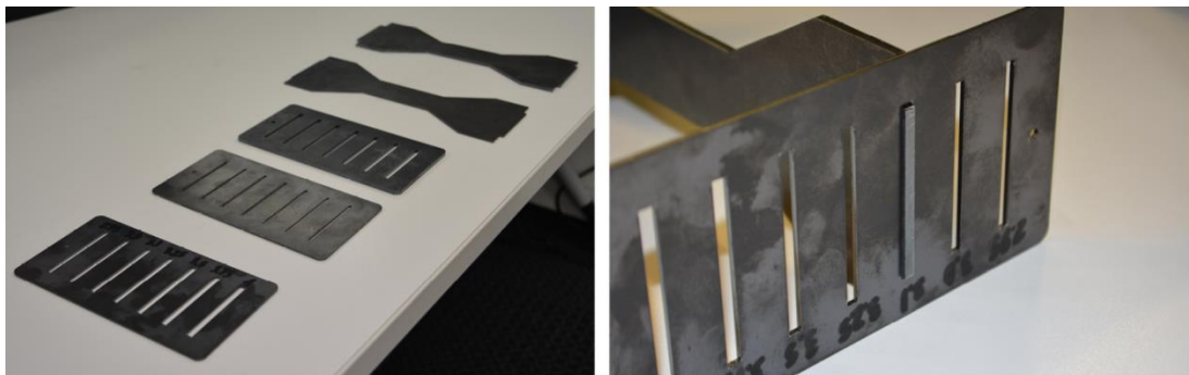
Figure 33. Prototype tab and slot components, laser cut in 1.6 and 3mm mild steel sheet
