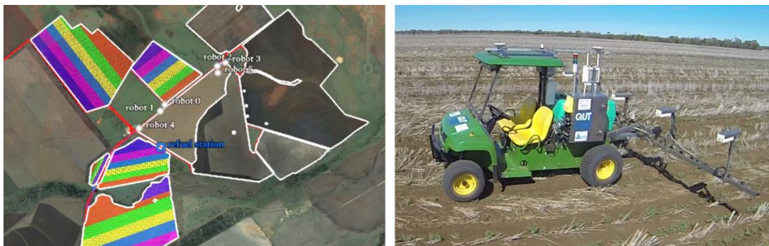
Figure 12. Video image of fleet cooperation around a farm (courtesy of ACFR) and the AgBot I undertaking autonomous driving and obstacle avoidance trials.
