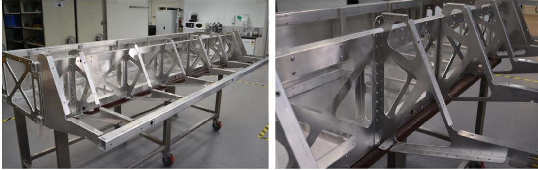
Figure 42. Depicts the frame structure across the front section of the implement unit.
