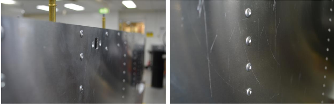
Figure 78. Dome head rivets using in the Implement Unit assembly.
