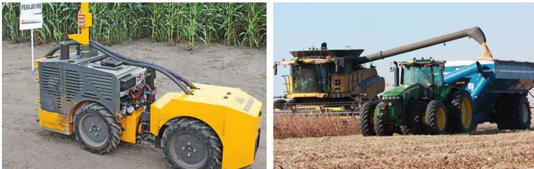
Figure 8. Rowbot [43] and Kinze autonomous grain cart [44]. Image copyright resides with the cited authors.
