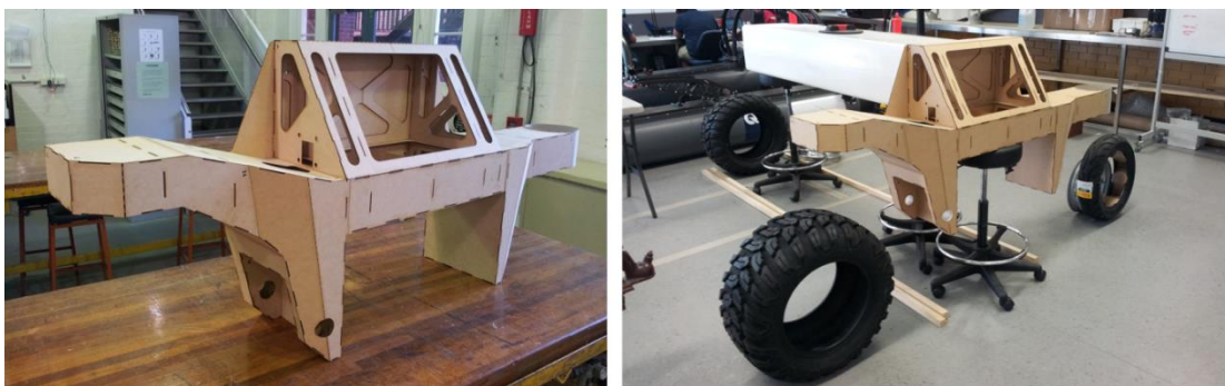
Figure 35. The completed POP prototype chassis ready for testing (left image) and the prototype in-situ (right image).
