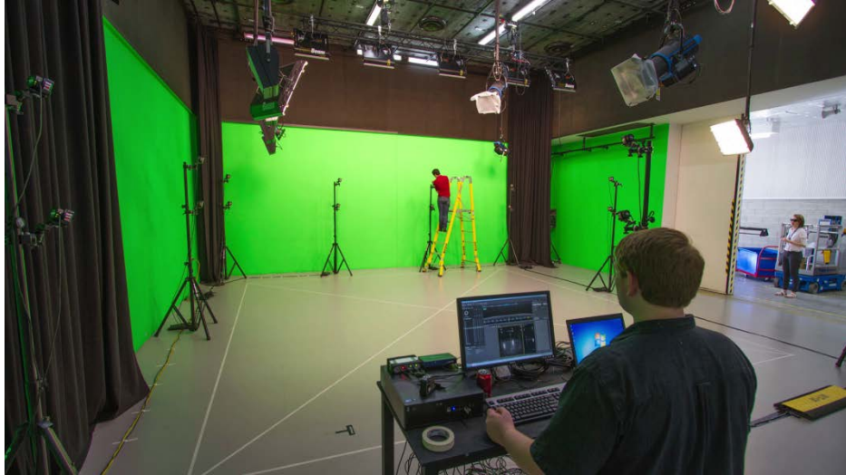
Figure 6. Optical motion capture system temporary setup at QUT
