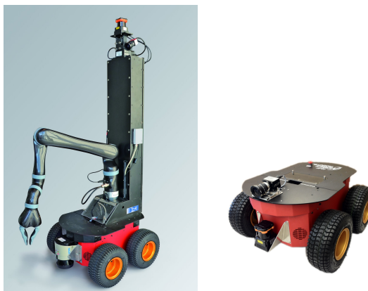
Figure 1. : Left: The mobile manipulator robot AMPARO. Right: The scout robot used for visual detection of infrastructure modules.
