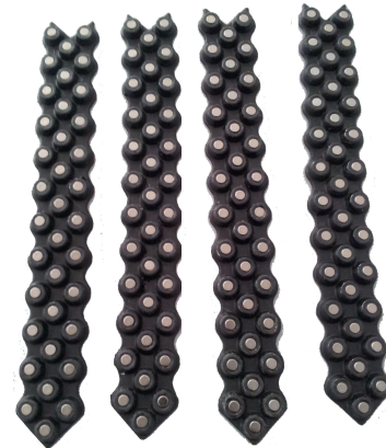
Fig. 5. New flexible concept for the magnet-wheel integration, based on polyurethane casting.
