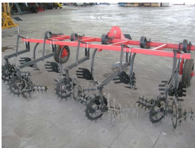
Fig. 1: Cultivator KON – 2.8 M, a rotational weed harrow
